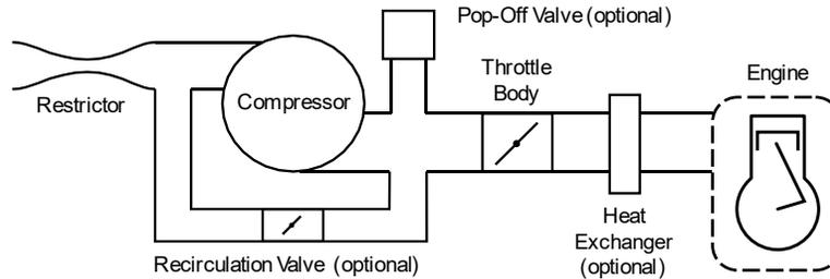
IC.2.4.3 The maximum restrictor diameters at any time during the competition are:
