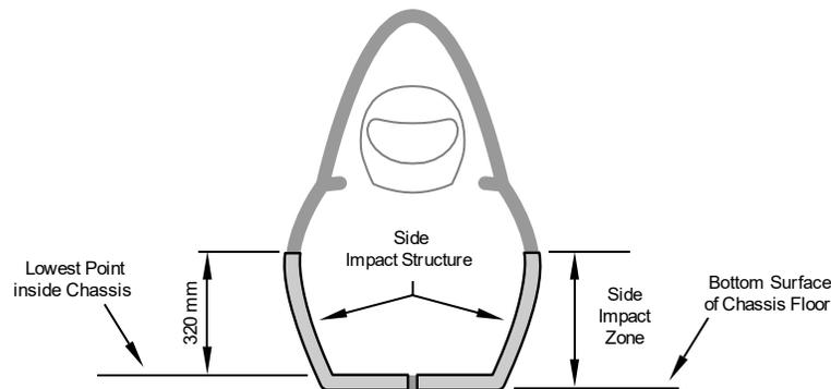
F.7.6.2 The Side Impact Zone must have a Buckling Modulus (EI) equal to three (3) Steel Tubes (F.3.2.1.e) that it replaces.
