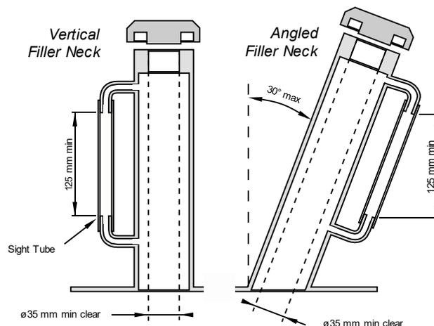
IC.5.4.5 **Fuel Level Line** - A permanent, non movable fuel level line must be located between 12 mm and 25 mm below the top of the visible portion of the sight tube.
