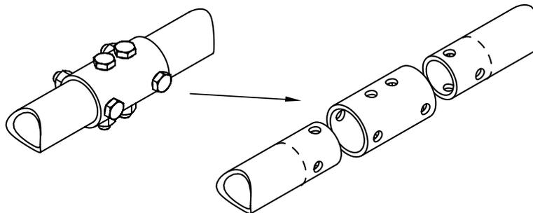
F.5.10.6 For Sleeved Butt Joints, the sleeve must:
