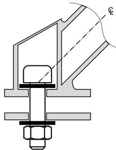
F.7.9.7 No crushing of the core is permitted
