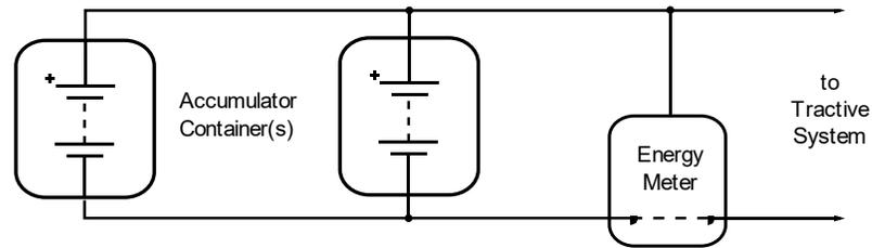
EV.6.1.4 All Accumulator Segments and/or Accumulator Containers (including spares and replacement parts) must be identical to the design documented in the ESF and SES
