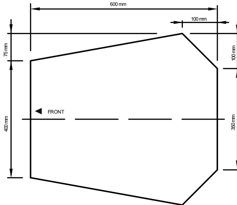
T.1.1.2 The template will be held horizontally, parallel to the ground, and inserted vertically from a height above any Primary Structure or bodywork that is between the Front Hoop and the Main Hoop until it meets both of: ( refer to **F.6.4** and **F.7.6.1** )
